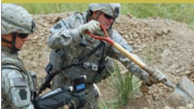
Two US soldiers equipped with an ICx Technologies Fido XT unit check vapours emanating from traces of explosive material. The system's sensitivity is said to be close to that of dogs. (US Army)
