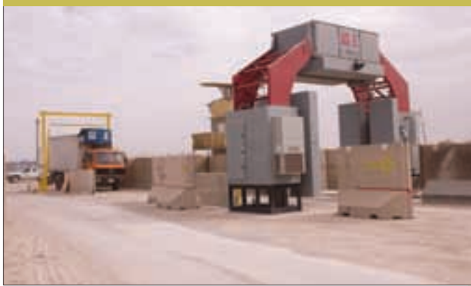
A vehicle scanner, produced by American Science and Engineering installed in Afghanistan, through which vehicles are typically driven at the speed of a man on foot. (Nato Consultation, Command and Control Agency)
