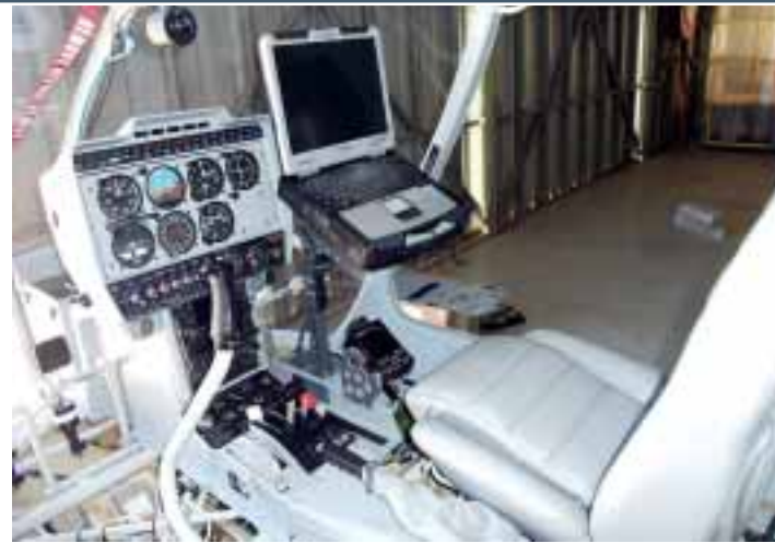
The Seeker cockpit showing the helicopter-like layout with centre instrument console. This is VH-SUA with the Wescam MX-10 video/IR sensor installed with its associated computer mounted in front of the operator's seat. Seabird
