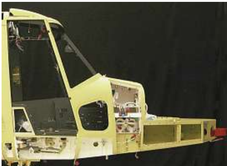
■ T101 in manufacture. Series production will adopt a 'pulse line' philosophy to improve skilling and reduce man-hours.
