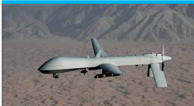
One of the most widely seen ISR assets in the Afghan skies is the MQ-1 Predator, different versions of which are in service with the American, British and Italian forces. (US Air Force)
