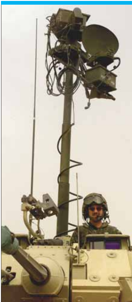
The mast-mounted radar of a Coyote armoured reconnaissance vehicle watches the perimeter of the Kandahar airfield. Those vehicles have proven to be valuable surveillance assets. (Canadian Armed Forces)
