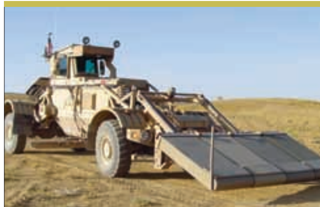
Niitek's Visor 2500 ground penetrating radar mounted on a US Army Husky. The system is modular and while the Husky can carry four modules, as seen here, lighter configurations are also being used. (Niitek)
