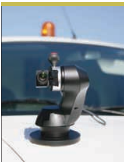
The Franco-German Institut Saint-Louis developed a change detection system that allows a vehicle operator to compare the video of a route itinerary with a recording taken earlier. (Institut Saint-Louis)
