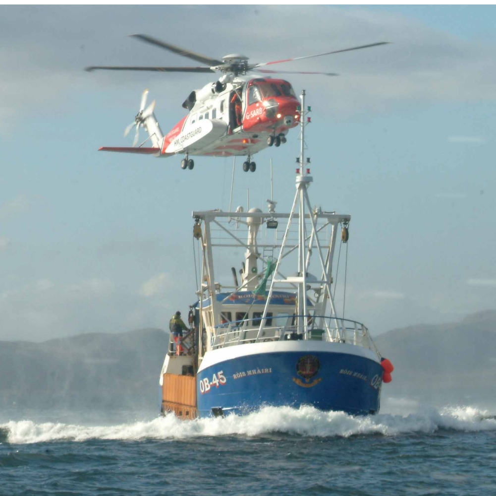
The Stornoway-based 'Romeo Bravo' practices winching operations from a fishing boat. Winching operations are facilitated by the pilot and winchman sharing a similar field of view.
