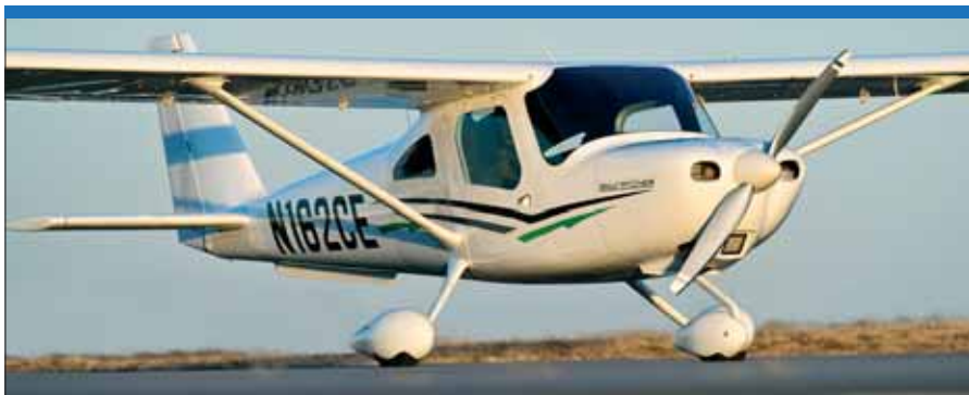
The screening of military student pilots may be performed on a sub-600 kg Light Sport Aircraft such as the Cessna 162 Sky Catcher, powered by a 75-kW engine and costing less than $ 150,000. (Cessna)
