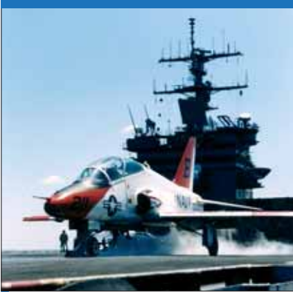
The Boeing T-45A/C Goshawk, developed from the BAE Systems Hawk and powered by a 24.2-kN Rolls-Royce Adour Mk 851 turbofan, was designed from the outset to include carrier training for US Navy pilots. (Rolls-Royce)
