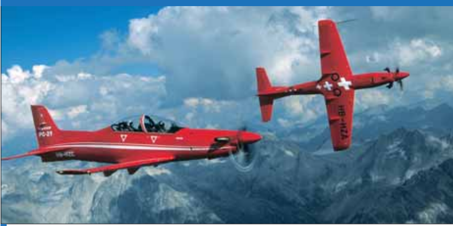
Probably the world's highest-performing turboprop trainer, the new Pilatus PC-21 is powered by an 1195-kW P&WC PT6A-68B engine. It has already been ordered by Singapore and Switzerland. (Pilatus)
