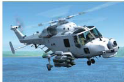
* Navy Wildcat looks the more different from existing Lynx, carrying updated sonar and anti-sub gear.
