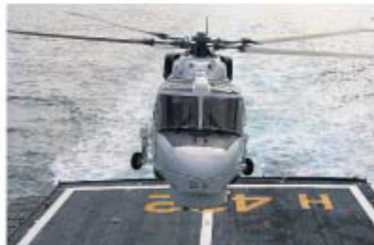
* Recently revised semi-rigid four-blade rotor assembly will be retained, vital for carrier-borne use.
