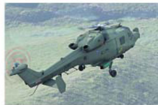
* New tail boom design and horizontal tail-plane are instant identifiers of the new Wildcat. Tail rotor new too.
