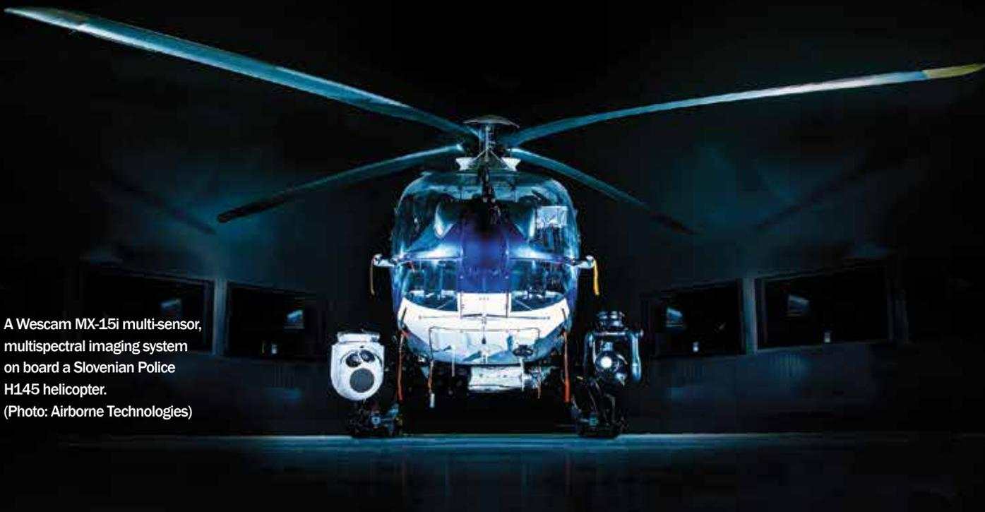
A Wescam MX-15i multi-sensor, multispectral imaging system on board a Slovenian Police H145 helicopter.
