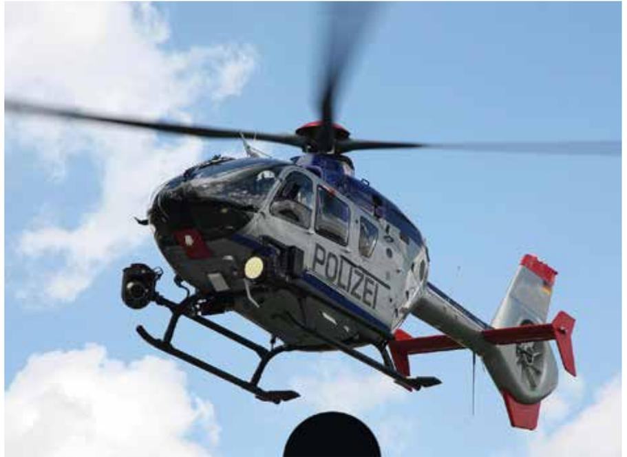
An H135 operated by the Saxony Police, with the FLIR Systems SAFIRE 380-HDc. (Photo: FLIR Systems)
