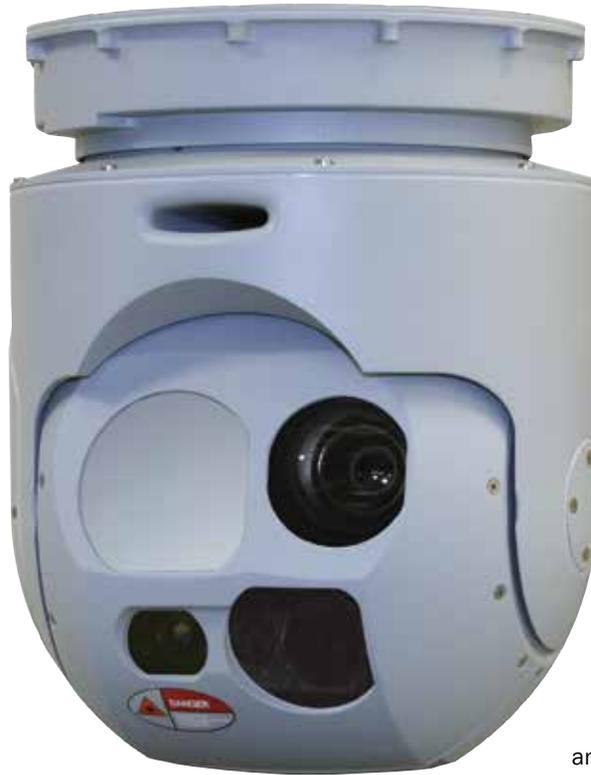
The MX-8 is a compact, multi-sensor, multi-spectral imaging system in a single LRU configuration. (Photo: L3 Wescam)
